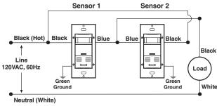
NOTE: Sensor 1 must be installed in a wall box that has both a LINE Hot. and a Ground connection. Sensor 2 must be installed in a wall box that has both a Load and a Ground connection.
