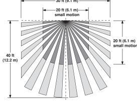
Small Motion = Dual Technology coverage. This also represents the maximum ultrasonic range coverage.
