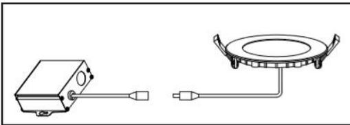
Hole Cut Size - Round 4":  $\text{Ø } 4 \frac{3}{16}" (106\text{mm})$
